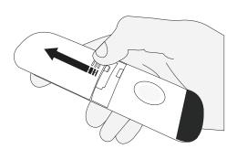
• Rotate the batteries around their axis (as shown in the illustration) and check for visual traces of soiling.
