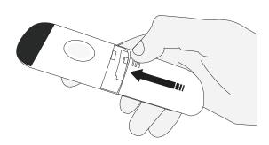
Clean the contacts of the remote control with a small amount of special cleaning agent (e.g. KONTAKT 60) using a cotton swab, cotton swab or soft cloth.
