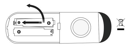
• Insert new batteries, making sure that the «+» and «-» polarities indicated in the compartment.
